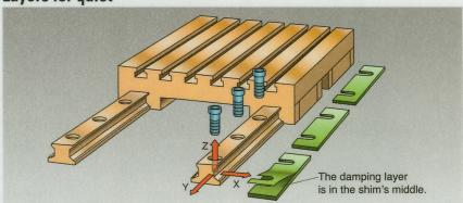
Laminated shims are made of thin sheets that can be peeled off to adjust thickness. Some varieties are embedded with electronic identifier chips that can report design specifications to handheld readers.
