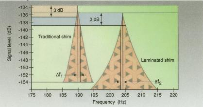
Shims designed for motion damping can absorb about 50% of vibration amplitude and reduce settling time by 50 to 55%.
